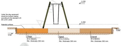
2.230 Colored rubber plates Thickness (According to the manufact of critical height of fall, based on test report Base: breakstone (fr.20-40 mm); Thickness 130-250 mm
