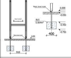
Play equipment areestablished with concreted steel foundation in equipment location. Equipment are suitable for use in two days after concreting, when the foundation are totally solid. During assambling there are not children allowed in area.
