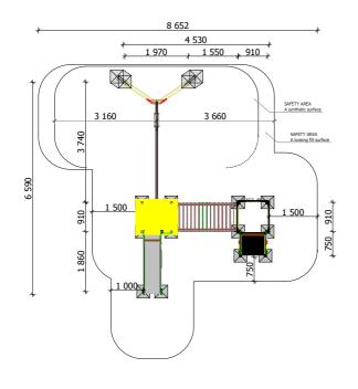
There must be in addition to 500 mm free of any obstacles in the swing direction to the rubber surface area.
