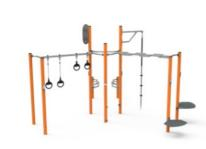
The snake ladder is made of hot-dip galvanized s235 steel with the following dimensions Ø38 x 4mm. The steel surfaces are hot dip galvanised inside and outside with lead free zinc. The galvanisation has excellent corrosion resistance in outside environments and requires low maintenance.
