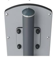
Steel posts are made of Ø101,6 x 2,0mm pregalvanized steel tube. The posts are powder coated .Tops of posts are sealed with plastic caps (PA6). Footings for surface installation are manufactured from Carbon steel with hot-dip galvanized surface according to ISO1461.
