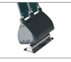
The rocking movement back and forth is controlled by a heavy duty scaled double rubber torsion spring element. The rubber element ensures a safe movement and reduces speed towards the tower platforms. The base cover of molded PE material with high impact resistance.
