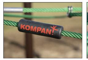
Ropes are made of UV-stabilized PES rope strands with inner steel cable reinforcement. The polyester wrapping is inductively melted onto each strand to obtain excellent wear and tear resistance.
