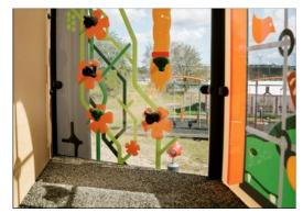
High-quality polycarbonate with a thickness of 15mm. The graphic prints are added by a unique multi-layer print process where the inner layer is the image and outer transparent layer functions as protection. Both PC panel and the water-based lacquer are UV stabilized to prevent fading.
