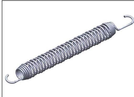
All 72 springs are made of stainless steel to ensure durability and excellent corrosion resistance. The steel wire is 3,2 mm thick and the last five windings are cone shaped to ensure long lifetime of the jumper.
