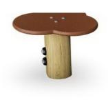
The steps are made of 21,5mm thick plywood made from alder and pine wood. Both sides are covered by 2 layers of phenolic film with anti slip net pattern. All cutting edges are sealed with paint to ensure long lifetime.
