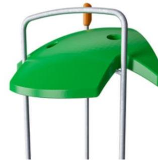
The ELEMENTS roofs are made of recyclable PE with a minimum wall thickness of 5mm to ensure high durability in all climates around the world. The steel pipes are hot dip galvanised inside and outside for maximum durability.
