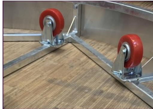
The roller system is designed with a fully closed lifetime lubricated center bearing supported by 10 wheels with a diameter of 125mm. The outer wheels ensures a smooth rotation under heavy load.
