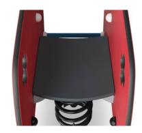
Seat is made of Ekogrip™ panel that consist of a 15mm thick PE base with 3 mm top-layer of soft rubber with a non-skid effect.
