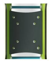
Seat is made of Ekogrip™ panel that consist of a 15mm thick PE base with 3 mm top-layer of soft rubber with a non-skid effect.
