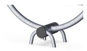
The rocking movement over axis is made by heavy duty scaled ROSTA torsion spring element. The ROSTA element works without any noise and requires low maintenance.
