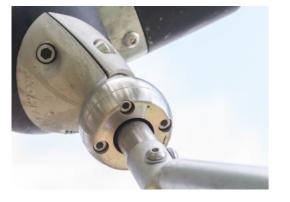
Bearing systems in heavy duty design in a maintenance free construction. All steel bearings are fully closed and lifetime lubricated. Coloured steel components has a base of hot dip galvanisation and a powder coated top finish. This provides an ultimate corrosion resistance in all climates around the world.
