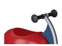
Handles are made with a moulded PP insert and an outer layer of soft TPV rubber. The handles are attached to the pipe with a galvanised steel inlay to ensure strength and durability.
